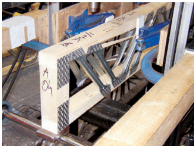
PICTURE: SPACEJOIST STRENGTH TEST
