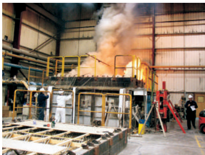
PICTURE: SPACEJOIST FIRE TEST
