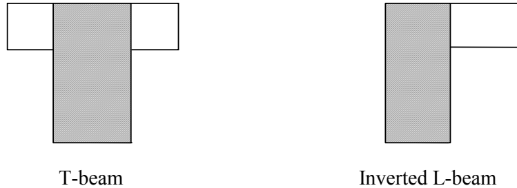
Figure 8.1 Rectangular area for the calculation of I_g (area shown shaded)
