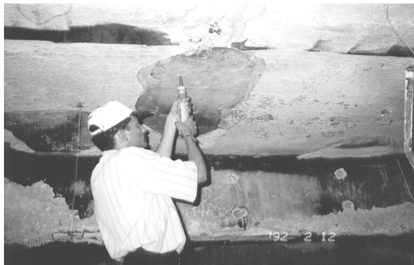
Figure 4.12 Use of Schmidt rebound hammer in a slab of building damaged by fire
