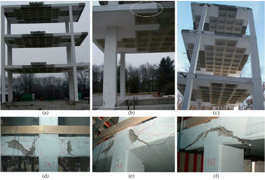
Plate 5 Flat slab frame after pseudodynamic test at the ELSA laboratory of the JRC: (a) side parallel to loading; (b) hinge in slab in positive (sagging) bending and plastic hinges at column base; (c) side at right angles to loading, with slab damage around connections; (d) edge slab-column connection, 1st floor; (e) edge slab-column connection, 2nd floor; (f) edge slab-column connection, 3rd floor (pictures (d)–(f) courtesy F. Taucer, JRC). (See also Figure 2.17 on page 107)
