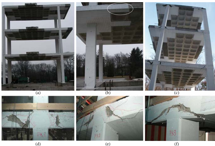
Fig. 2.17 Flat slab frame after pseudodynamic test at the ELSA laboratory of the JRC: (a) side parallel to loading; (b) hinge in slab in positive (sagging) bending and plastic hinges at column base; (c) side at right angles to loading, with slab damage around connections; (d) edge slab-column connection, 1st floor; (e) edge slab-column connection, 2nd floor; (f) edge slab-column connection, 3rd floor (pictures (d)–(f) courtesy F. Taucer, JRC). (See also Colour Plate 5 on page 719)
