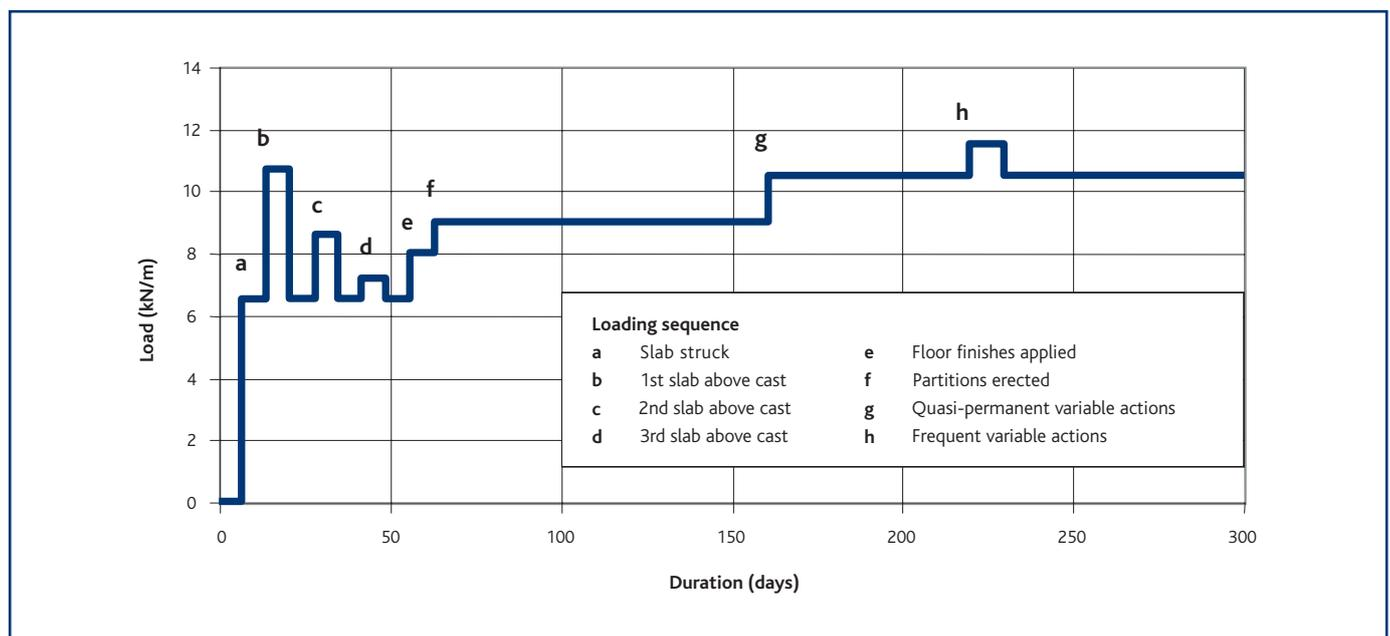
any of the earlier load stages. If, however, an earlier stage proves critical, the  $\zeta$  value at that stage should be carried forward to all subsequent stages.
