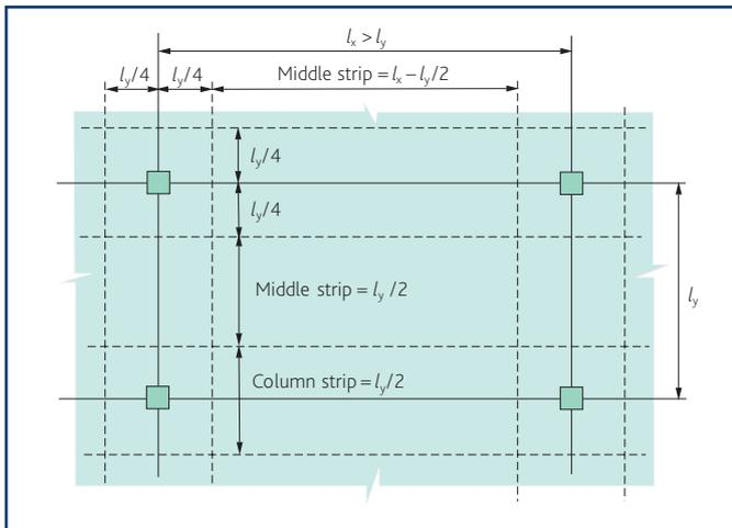
At internal columns, unless rigorous serviceability calculations are carried out, top reinforcement of area  $0.5 A_t$  should be placed in a width equal to the sum of 0.125 times the panel width on either side of the column.  $A_t$  represents the area of reinforcement required to resist the full negative moment from the sum of the two half panels each side of the column. It is also advisable to apply this requirement to perimeter columns as far as is possible.
