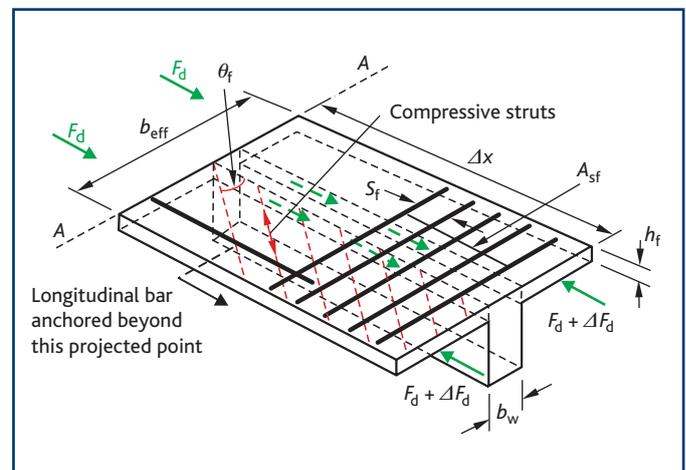
the interface of the flange and web can be resisted by the transverse reinforcement in the flange. The position of the neutral axis should be determined, and then the area of reinforcement can be calculated depending whether it lies in the flange or web (see Figure 11).
